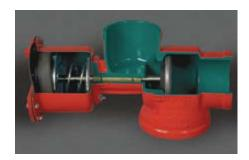
Our patented cast-iron backwash valve has the lowest pressure drop in the industry and is designed to be 100% field serviceable with basic hand tools. Valves feature non-corrosive stainless steel shafts, brass bushing, durable molded polyurethane seals, fusion epoxy lining, and a grease fitting for valve shaft lubrication.
